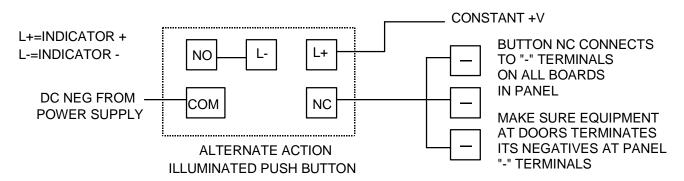
FIG. 8: FIELD INSTALLATION OF EMERGENCY RELEASE BUTTON
